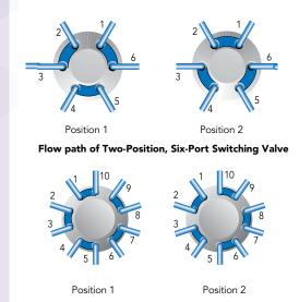
Flow path of Two-Position, Ten-Port Switching Valve
