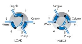
Flow path of Two-Position, Six-Port Injection Valve
