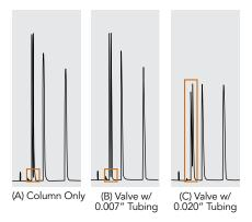
**Conclusion:** These sequential chromatograms show the effect of adding volume to the flow path through the addition of components.
