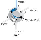
Flow path for the typical dual mode injector
