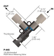
For fine control of fluid flow rates, Micro-Metering Valves can reduce outgoing flow to as low as 3.5 µL/min\*. These needle valves are perfect for use with peristaltic pump fluid-transfer applications, mass spectrometry, and fraction collection.
