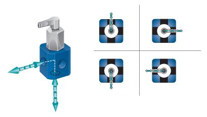
Distribution valves are used to direct fluid to a number of locations. 2-, 3-, 4-, 6- and 8-port valves are available with a distribution type valve plug. The 2-, 3-, and 4-port distribution valves are available in HV, HVP and HVX body styles. The 6- and 8-port valves are available only in the HVX body style. The flow configuration drawings show the possible fluid flow paths for a 4-port valve with a distribution type plug.
