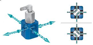
Loop valves are used to direct and redirect fluids. 4-, 6-, or 8- port valves are available with a loop type valve plug. The 4- port valve is available in HV, HVP and HVX body styles. The 6- and 8-port valves are only available in the HVX body style. The flow configuration drawings show the possible fluid flow paths for a 4-port valve with a loop type plug.
