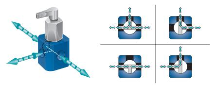
Flow valves are used to direct or redirect fluids. 2-, 3-, and 4-port valves are available with straight through (180°), 90°, or "T" type plugs for seven different valves. All seven flow configurations are available as HV, HVP and HVX valves. The flow configuration drawings show the possible fluid flow paths for a three port flow valve with a "T" type plug.
