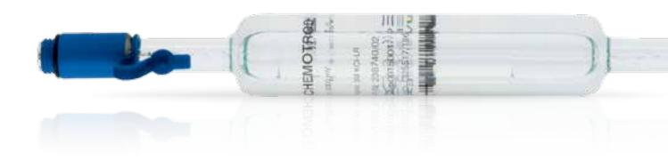
The ChemoTrode ORP is the most robust sensor to measure the oxidation-reduction potential in demanding applications in pharmaceutical and chemical industries. The ChemoTrode has a refill hole which allows refilling the electrolyte and pressurization of the reference electrolyte. Its Everef-F reference cartridge ensures that the reference electrolyte remains free of silver and precipitation of proteins.
