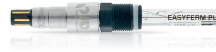
The EasyFerm Plus ORP sensors are designed to withstand demanding applications in pharmaceutical and chemical industries. It is supplied with a prepressurized electrolyte which prevents the diffusion of sample into the sensors. The Everef-F reference cartridge ensures that the Phermlyte reference electrolyte remains free of silver and precipitation.
