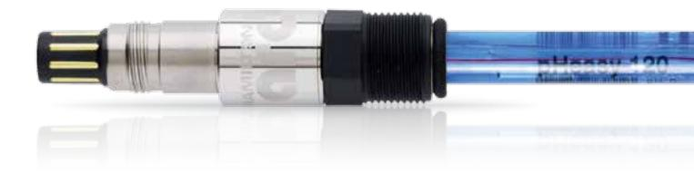
The pHeasy is one of the first pH sensors with a built-in lifetime monitoring without calibration. The second reference electrode helps to detect reference problems and indicates when the sensor has to be changed. It is designed for various applications where monitoring the longterm stability is appreciated like in the chemical industry or in wastewater treatment.
