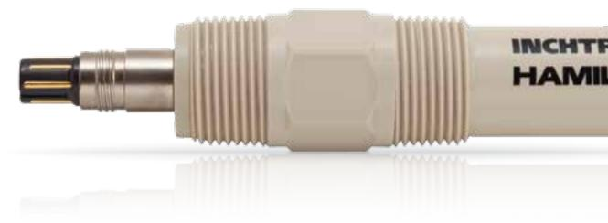
The InchTrode sensors are designed to measure pH in demanding applications in the paper making as well as in the chemical industries. The Single Pore liquid junction guarantees best and fast measuring results because of direct contact between the sample and the Polisolve electrolyte.
