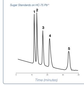
Column: HC-75 Lead Form, 5  $\mu$ m, 7.8 mm x 305 mm
