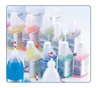
Top-down traceability: With Hamilton, the pH value of the DuraCal buffer is determined by a comparison with two secondary
