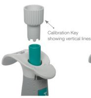
3. Insert the calibration key. Each vertical line on the calibration key is approximately 0.2% of the pipette's total volume.
