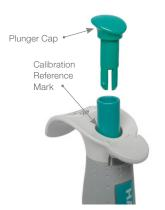
2. Locate the calibration reference mark and remove the plunger cap.
