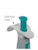
1. Remove the calibration label. Initial and date a new calibration label and place on the pipette.
