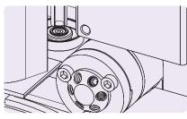
4. Install the stator head, then the stator face. Replace the stator screws, tightening them evenly and carefully.
