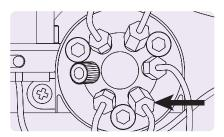
1. Disconnect the seat capillary from the injection valve (port 5).
