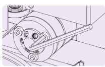
1. Remove the capillaries from the stator face. Remove the stator screws with a 9/64" Allen wrench.
