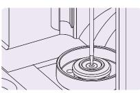
4. Situate the needle approximately 2 mm above the seat using the "Needle Up" function. Ensure the needle is aligned with the seat.
