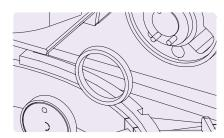
3. Remove and replace the rotor seal (and the isolation seal, if necessary).
