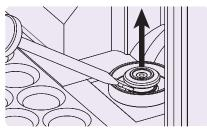
2. Use a small, flat screwdriver to ease out the needle seat.
