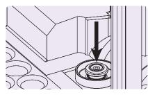
Insert the new needle-seat assembly.
