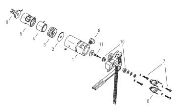
5975/5973 MSD Electron Impact (EI) ion source assembly
