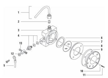
FPD ignitor and heat shield assembly
