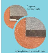
Agilent's non-stick septa are plasma treated, eliminating chemical bleed and contamination caused by foreign substances, like the damaging talcum powder used by other suppliers.
