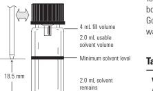
Needle tip position when withdrawing solvent
