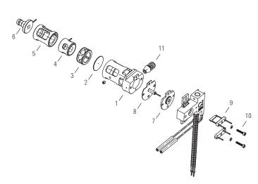
5975/5973 MSD Chemical Ionization (CI) ion source assembly
