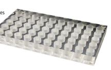
**9504R-01** 1/each Racks, acrylic, for 15mm vials. 175.8 x 115.5 x 20mm, 40 cavities 15.1mm diameter.
