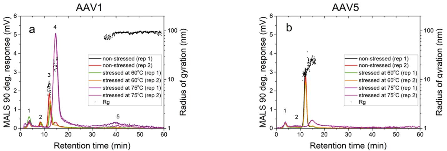
Figure 5 a and b: 90° light scattering signal-based fractograms and radius of gyration ( $R_g$ ) profiles of two serotype AAV samples at room temperature and stressed at 60°C and 75°C, a) AAV1, b) AAV5, inserted numbers represent different components, 1 and 2: fragments, 3: monomer, 4: oligomers, 5: larger aggregates.
