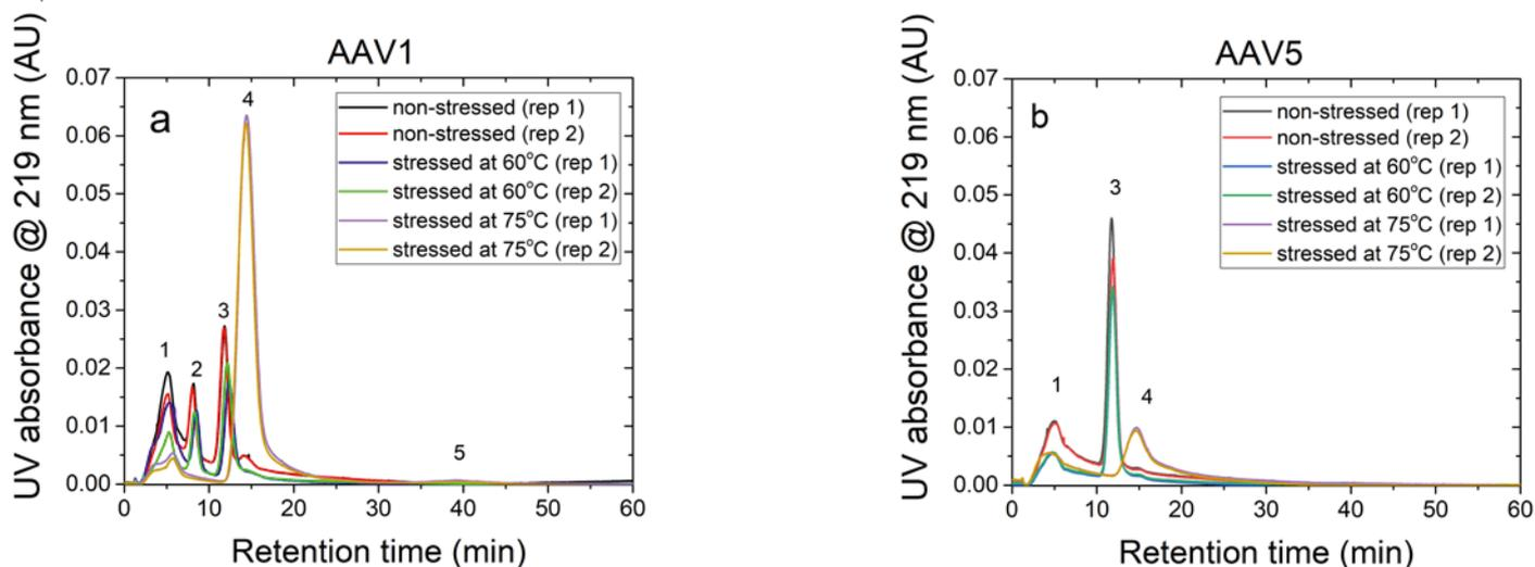
Figure 4 a and b: UV absorbance at  $\lambda = 219$  nm versus retention time of two serotype AAV samples at room temperature and stressed at 60°C and 75°C, a) AAV1; b) AAV5, inserted numbers represent different components, 1 and 2: fragments, 3: monomer, 4: oligomers, 5: larger aggregates.
