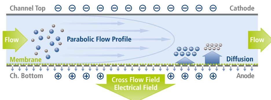
Figure 1. Schematic representation of an Electrical Asymmetrical Flow FFF channel used for analysis of negatively charged particles where the accumulation wall (membrane) was chosen to be the anode. The polarity of the channel walls can be changed readily according to the particle charge type and desired direction of the electrical field.
