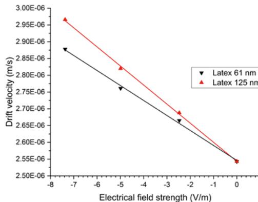
Figure 5: EAF4-MALS fractograms of the investigated nanoplastics particle mixture obtained for four different electrical field strengths (left). Differential velocity versus electrical field strength plot to determine the electrophoretic mobility of the two nanoplastic particles in the mixture (right).
