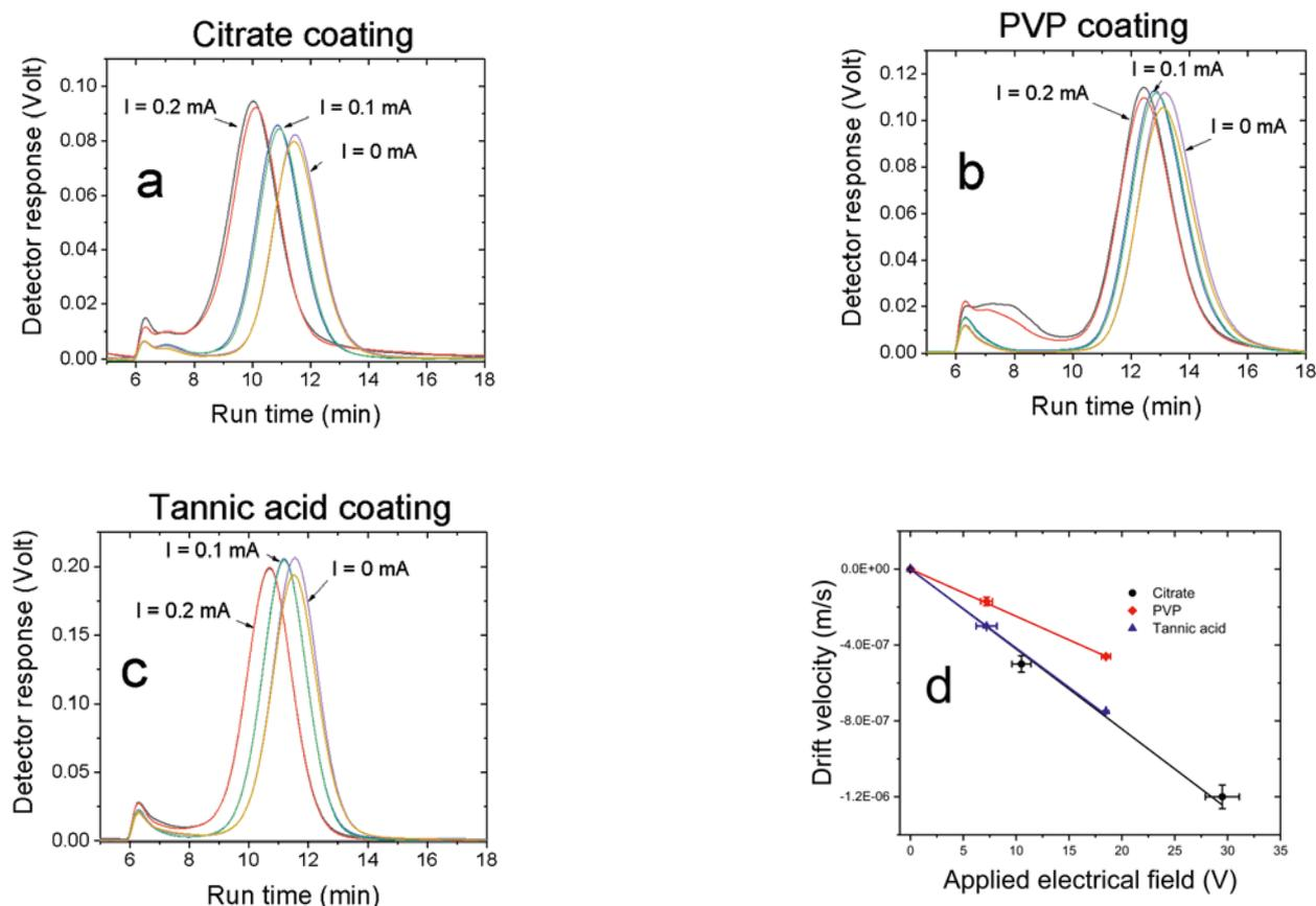
Figure 2. UV-based fractograms of 50 nm Ag NPs with different surface coatings. a) citrate coated, b) PVP coated, c) tannic acid coated, d) plot of net drift velocity versus applied electrical field.
