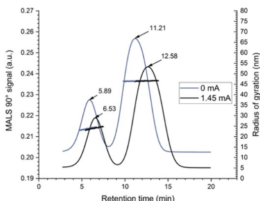
Figure 4. EAF4-MALS fractograms of the investigated nanoplastics particle mixture with and without application of an electrical field (black and blue graph, respectively). The blue and black dotted lines display the radii of gyration obtained from MALS indicating no influence of the electrical field on the particle size.
