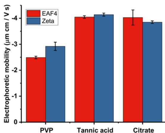
Figure 3. Comparison of the electrophoretic mobility values obtained from EAF4 and zeta potential measurements.
