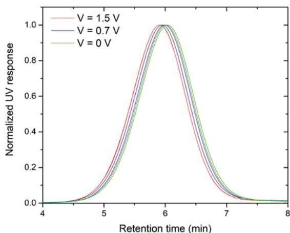
Figure 6. NIST mAb retention time shift with applied electrical field (recorded in voltage mode).
