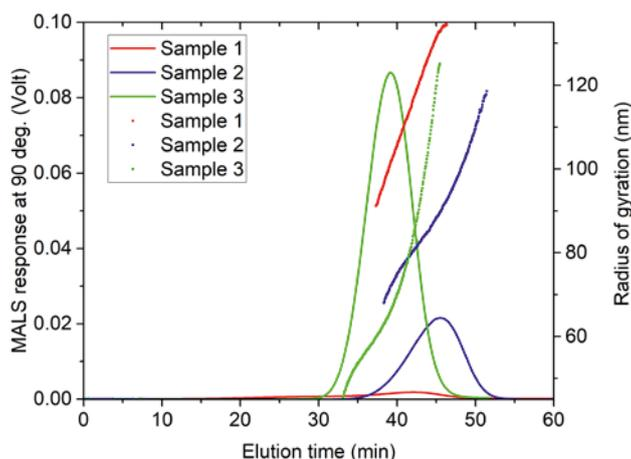
Figure 3: Fractogram for three polyacrylate samples separated by TF3. The curves correspond to MALS response at 90°; the dots are the measured radius of gyration at each time point.
