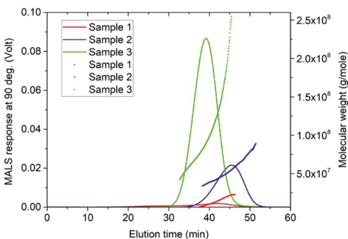
Figure 2: Fractogram for three acrylate samples separated by TF3. The curves correspond to MALS response at 90°; the dots are the measured molecular weight at each time point.
