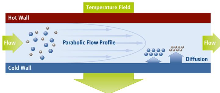
Figure 1: Schematic of the TF3 channel.
