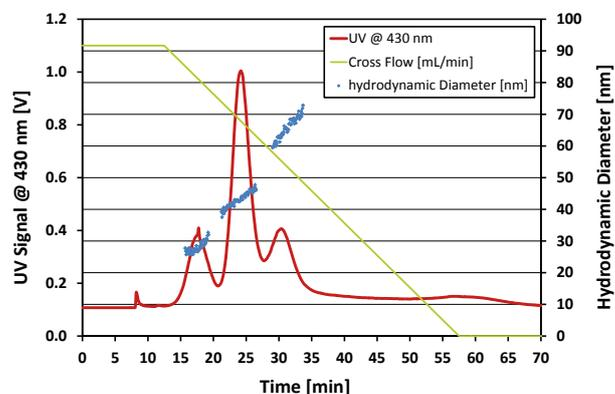
Figure 3: AF4-DLS fractogram of a 1:1:1 (w/w) mixture of AgNP (20 nm, 40 nm, 60 nm).
