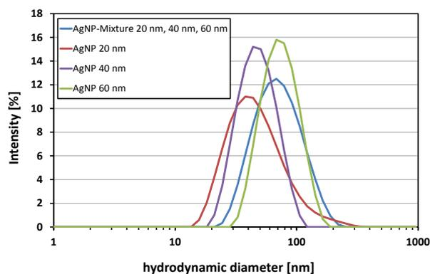
Figure 2: Comparison of intensity-based particle size distributions for single AgNP and AgNP in a 1:1:1 (w/w) mixture obtained from DLS in batch mode.
