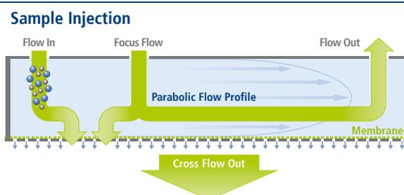
Figure 2: Schematic illustration of High Volume Injection in AF4.
