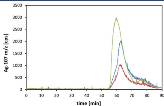
Figure 6: AF4-ICP-MS fractograms of AgNP spiked in Rhine water (628 ng/L, blue trace; 321 ng/L, red trace) and ultrapure water (1037 ng/L, green trace).
