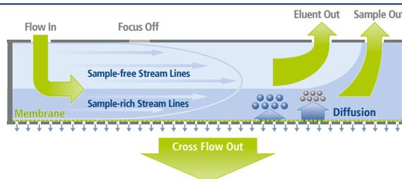
Figure 4: Schematic illustration of S3 in AF4.
