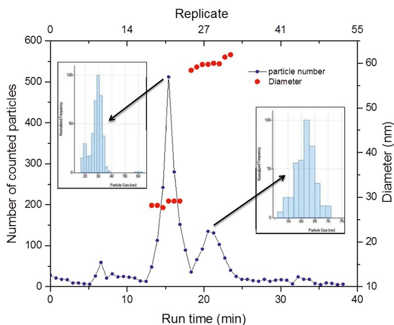
Figure 2. Particle number-based fractogram of the mixture of 30 nm and 60 nm Au gold nanoparticles obtained by AF4-spICP-MS. The red circles represent the average replicate diameter measured by spICP-MS. The shown histograms representing the particle size distribution at the respective peak maxima are directly obtained from the Agilent MassHunter Workstation software.
