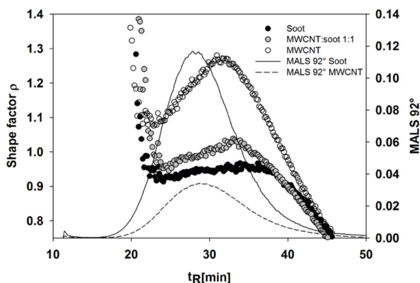
Figure 1: Fractograms obtained by AF4-MALS with shape factor  $\rho$  (symbols) for equal mass injections ( $5 \mu\text{g}$ ) of a pristine long MWCNT, soot and a 1:1 mixture of both. Lines show the  $92^\circ$  MALS signal of pure soot (solid) and pure MWCNT (dashed).
