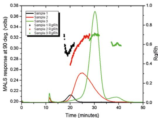
Figure 3. The ratio of  $R_g/R_h$  plotted across each peak in the fractogram.
