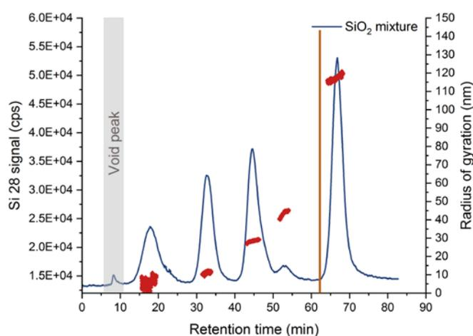
Figure 3: Obtained AF4-MALS-ICP-MS fractogram indicating five different silica particle size populations in the sample (blue trace:  $^{28}\text{Si}$  signal; red dots: Radius of Gyration from MALS; orange line: lower size limit of spICP-MS).
