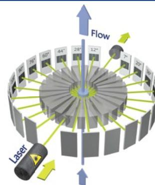
Fig. 3: Principle of MALS detection.
