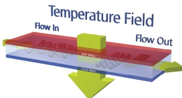
Fig. 1: Principle of Thermal Field-Flow Fractionation.
