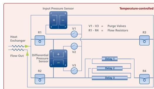
Fig. 4: Principle of Viscosity Detection.
