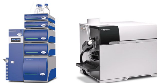
Figure 1: Postnova AF2000 MT and Agilent 7900 ICP-MS.
