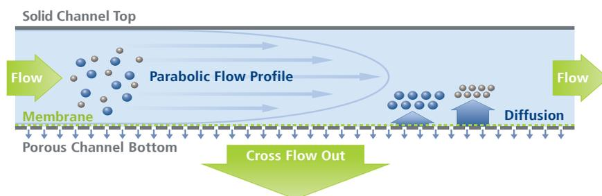
Figure 2: Schematic of the AF4 separation principle.
