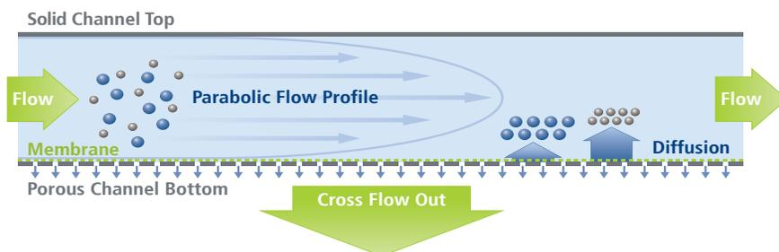
Figure 2: Schematic of the AF4 separation principle.
