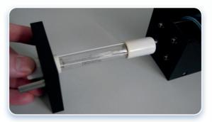
The UVD can be used for flow rates from 0-10 mL/min and is ideal for any aqueous based eluents which show acceptable UV absorption properties. The only spare part is the UV lamp which needs a replacement after a certain operation time (approx. 8000 hours), depending on use and switching cycles. The status of the UV light source is displayed via LED at the front cover of the UVD module.
